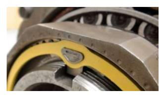
Retainer Tab Inserted Correctly in Nut.
