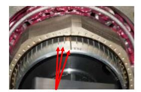
Dots on Nut Face NOT Aligned with Hash Marks on Circular KeyFinder.
