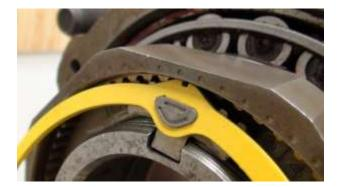
Retainer Tab Entering Groove in Nut.
